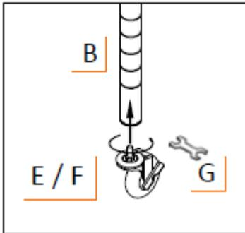
Warning: Tighten CASTERS (E & F) to BOTTOM POLES (B) completely. Failure to do as instructed could result in the caster stem breaking.
