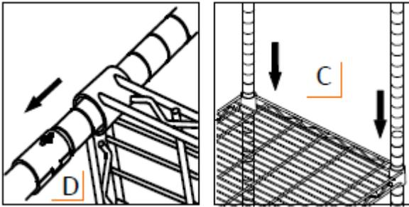
Note: The level side of the SHELF (C) is the TOP side (the TRINITY logo on the corner cylinders should be right-side up).
