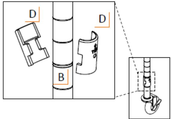
Note: For stability, the lowest SLIP SLEEVES (D) should be installed ***no higher*** than the 3rd indentation from the caster end of the BOTTOM POLES (B).
